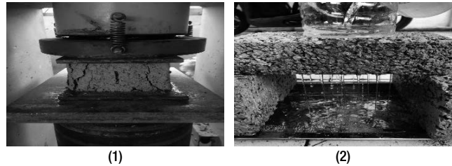
Fig. 1. Type A (1) Compressive strength, and (2) Infiltration
